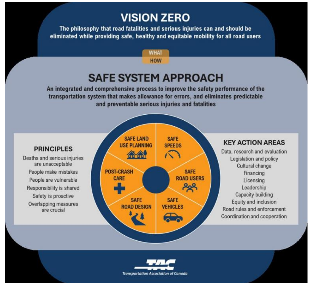
Figure 1: Vision Zero and the System Approach Framework (Source: Transportation Association of Canada: Vision Zero and the Safe System Approach: A Primer for Canada (2023))
